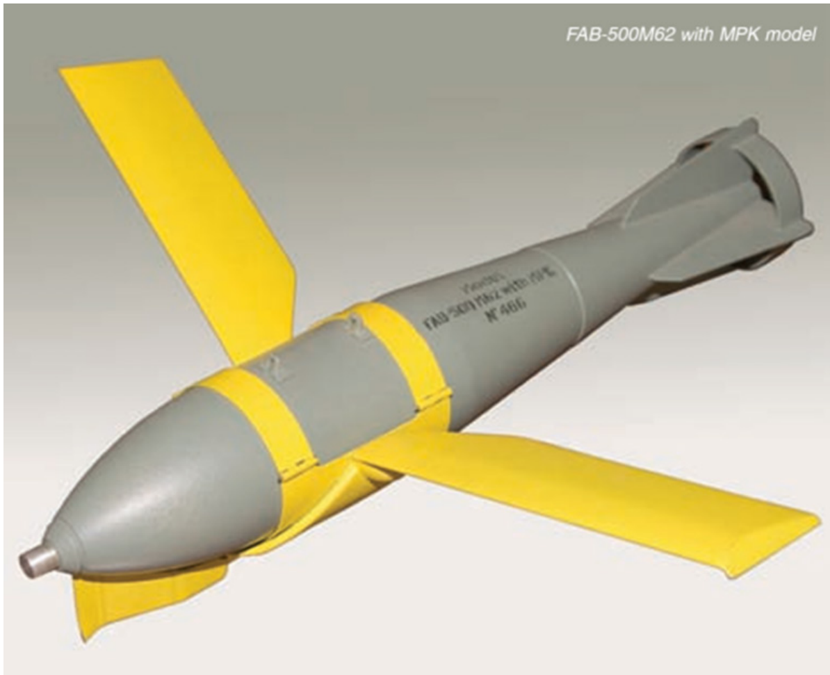
Figure 4: FAB-500M62 bomb with MPK model (Source: "Take-off", Feb. 2009, photo by Yevgeny Yerokhin)
