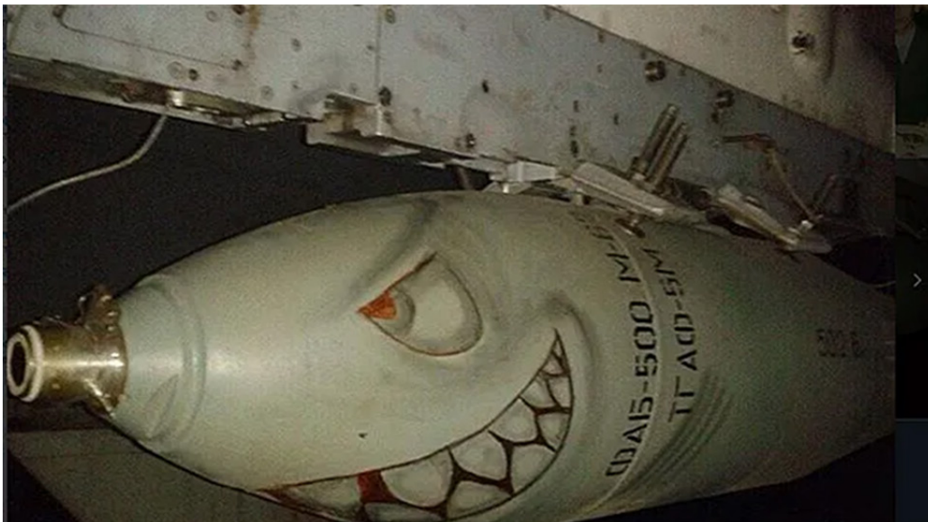
Figure 18: Rambler/TK Zvezda photo of FAB-500 M62 with painted shark and TGAФ-5M markings.
